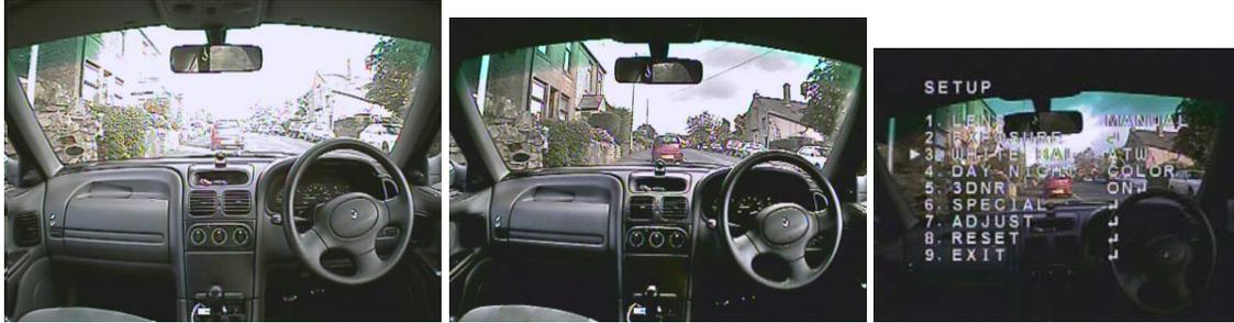
There are a few things to consider when setting up the dominator camera depending on where your camera is positioned and the surrounding light levels. The camera can be configured accordingly and to do this there is a joystick on the rear of the camera hidden under the screw cap on the rear. Remove the screw cap and press the joystick once to bring up the menu system (as an overlay image on your monitor or DVR screen). Move the joystick accordingly to navigate the menu options.
