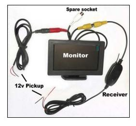
The camera is supplied with screw and self adhesive mounting options. The monitor has a self adhesive mount bracket but also included is some double sided Velcro which can be used on the rear of the monitor to enable other fitting locations. For product news, updates and accessories please visit www.4KamVU.com
